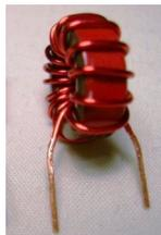
Figure 9. Filter Toroid Winding
