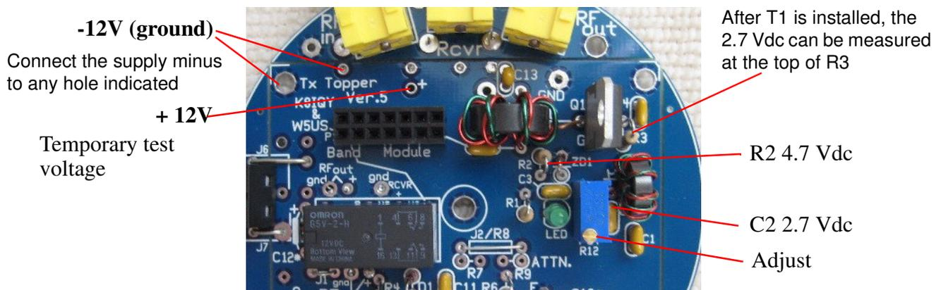
Figure 7. Gate Bias Test Connections
