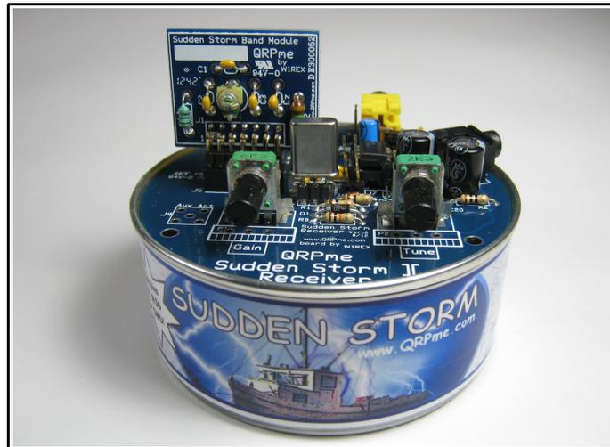
Mount the completed circuit board on the top of the tuna can using the 6-32 bolt & nut. The nut should be at the bottom of the can. You can now insert the SA612 chip, crystal and band module board. You are ready to operate!
