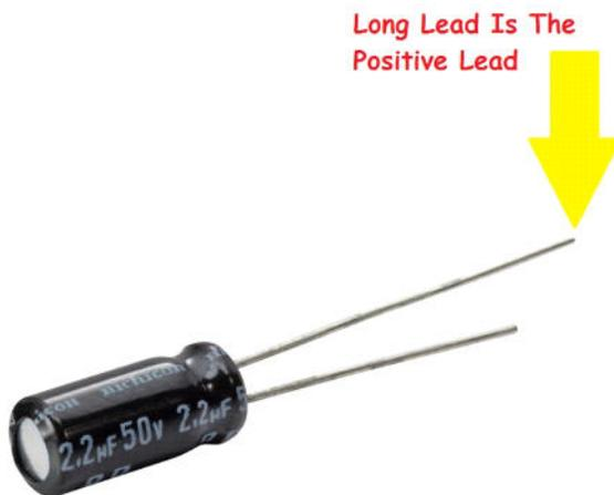
Install C3 and C5: 2.2uf (Electrolytic Capacitor)
