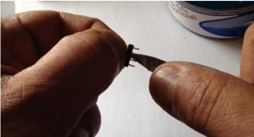
4 pin (2x2x.1") Molex dual row header cut in half and inserted.
