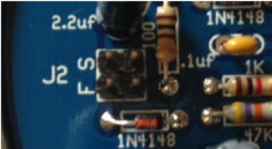
Place the Headers on J1 and J2. \*\*\* This is so to aid in securing the pins in place while you place a piece of tape on them so they will not fall out when you are soldering them \*\*\*
